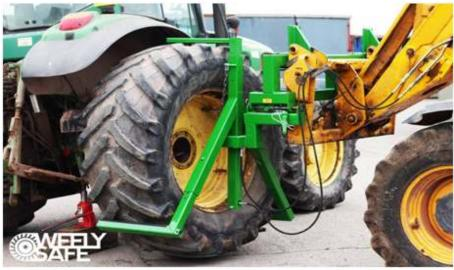
It is <u>Clean, Simple</u> and <u>Safe</u> to use, enabling the operator to remove, carry, store & refit most large tractor / combine wheels & tyres up to 2m in diameter either in a yard or even field situations. It will fit most tractor loader machines and telehandlers. With ever increasing wheel sizes and lone working situations, it is a must for every farm.
